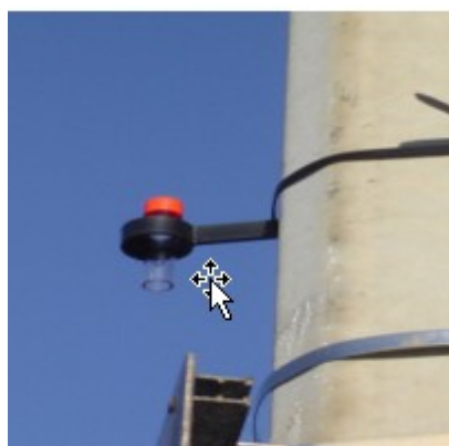
Monitoring of NO 2 , using both continuous (automatic) monitors and passive diffusion tubes
