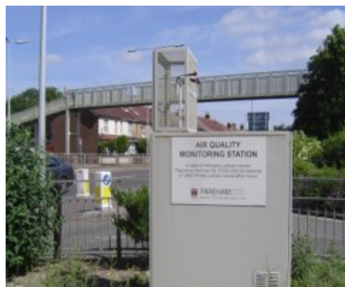
Monitoring of NO 2 , using both continuous (automatic) monitors and passive diffusion tubes
