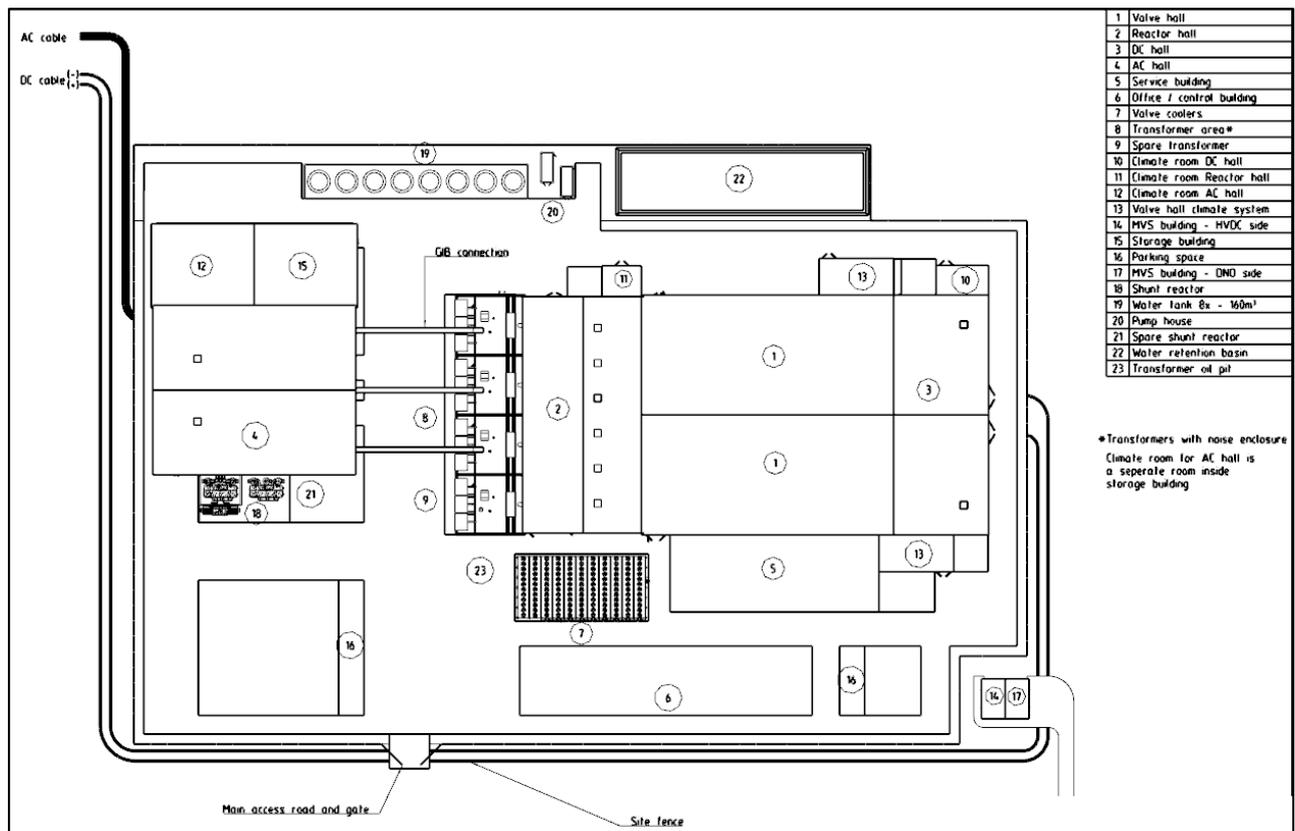
Figure 1– Detailed equipment layout of Daedalus HVDC station
