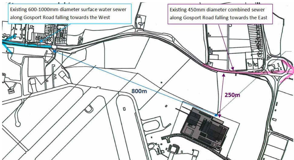
The closest connection is a 450mm diameter combined sewer approximately 250m north of the site to which there appears to be several existing manholes along Gosport Road where connection could be made. This sewer flows towards the east and across the roundabout however it is not clear where this sewer ultimately discharges.
