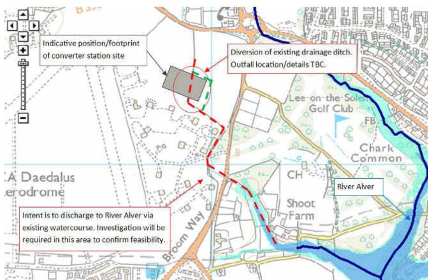
It should be noted that on another project in the Daedalus Enterprise Zone the surface water drainage layout suggests a very similar approach was adopted with attenuation, flow control and discharge to this watercourse.
