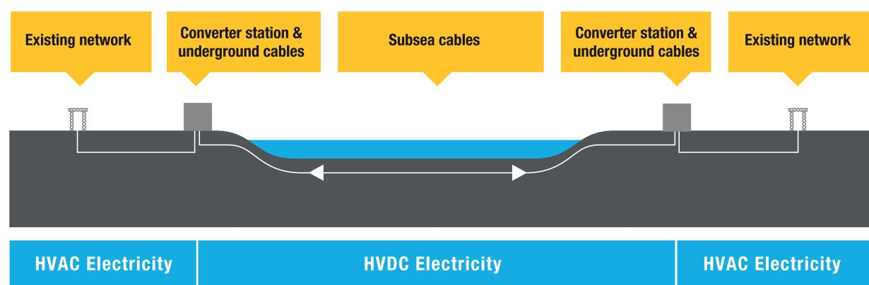
Being an island, Great Britain requires connections with other countries to be made using subsea cables. Differences between electricity transmission in Great Britain and continental Europe, as well as the distances involved, require using high voltage direct current HVDC.
