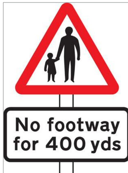
Figure 7.1: TSRGD diagram no. 544.1 'pedestrians in road ahead'
