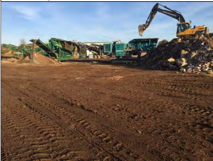
Photo 5: Aggregates screening and crushing
